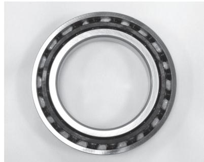
**Fig. 8.3** Turn by hand so that the grease is fully distributed in the bearing. While turning by hand, apply an adequate load to the inner ring
