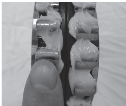
**Fig. 8.6 With fingers, spread the grease deposited on the outer surface of the rib on the cage**
