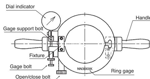
Mount the outer ring into the housing and then measure the outer ring raceway diameter. Place the cylinder gage, onto the bore surface of clearance adjustment gage and adjust it with the open/close bolt. Insert the gage into the outside diameter portion of the roller set in the inner ring as shown in Fig.8.17. Be careful not to damage the rollers.
