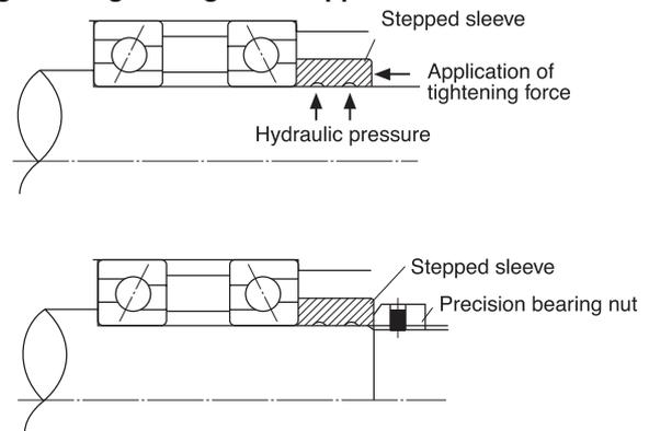
Tightening with a precision bearing nut (precision lock nut) provides a predetermined tightening force by controlling the bearing torque shown in Fig 8.11. When locking the bearing with a precision bearing nut, make sure that the squareness between the bearing surface and the shaft centerline is 3 μm or less so that adequate bearing accuracies are maintained.
