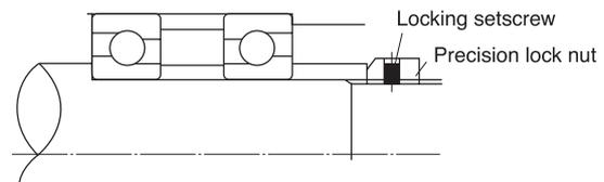
Because the thread face of the precision bearing nut, the thread face of the shaft and the bearing surface and nut constitute sliding surfaces, the correlation between tightening torque and tightening force will vary depending on the friction coefficient. Therefore, the nut needs to be
