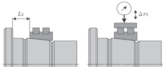
(c) To adjust the bearing clearance to a predetermined target value ( $\delta$ ) after mounting, determine the spacer width  $L_n$  with the following formula (Value  $f$  in the formula refer to Table 8.3)
