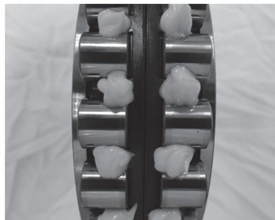
**Fig. 8.5 Apply grease to the outer side of the rollers, and while turning the rollers with fingers, spread the grease to the inner ring (outer ring) side**
