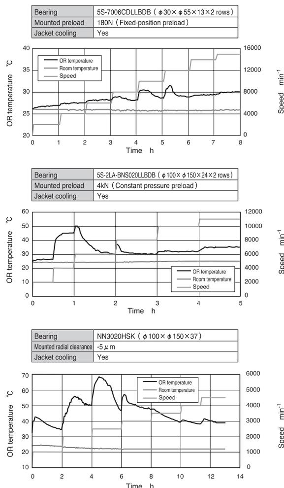
**Fig. 8.8** The bearing is run for several minutes up to about the maximum allowable speed limit of the bearing
